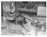
Operating clamping force: 500 daN (hand applied), 800 daN (mallet applied).
