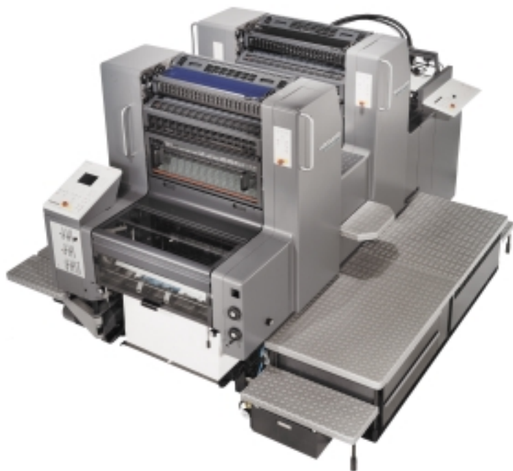
Two-colour offset printer with stirrup-shaped handles with pearl-brightness chromium plating.
