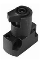
Base or Front Mounted. Manually turned. Tightened & released by hexagonal key. Spring return. Nominal Holding Force: 2000 daN
