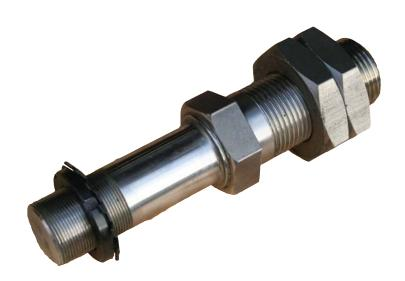
This range of cantilevered stub axles is designed to mount single wheels with ball or roller bearings, the lock nut and lock washer, or self locking nuts providing adjustment for opposed taper roller bearings.
