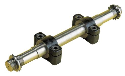
These axle assemblies are for mounting pairs of wheels fitted with ball or roller bearings, the lock nuts and washers, or self locking nuts providing adjustment for opposed taper roller bearings.
