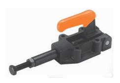
Plunger: Ground Steel. Locks at both extended & retracted ends of the stroke. Base: SG Iron Casting. Body mounting. Nominal Holding Force: 600 daN Weight: 0.45 Kg Supplied complete with: MB0840 Setscrew & nut.
