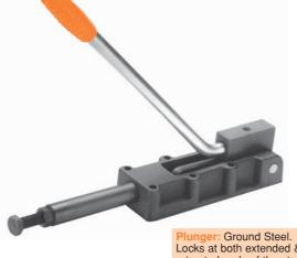
With 20 daN handle force the output force is: daN Fully retracted 1100 10 mm extended 180 20 mm 110 ,, 75 80 30 mm ,, 40 mm ,, 50 mm 82 ,, 100 100 60 mm ,, 70 mm ,, 80 mm 130 ,, 190 250 90 mm ,, 95 mm ,, 97 mm 310 ,, 99 mm , Fully extended 450 1210
