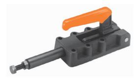
Plunger: Ground Steel. Locks at both extended & retracted ends of the stroke. Base: SG Iron Casting. Body mounting. Nominal Holding Force: 2500 daN Weight: 3.60 Kg Supplied complete with: MB1250 Setscrew & nut. See "Accessories" for other items.
