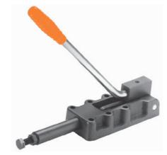
Plunger: Ground Steel. Locks at both extended & retracted ends of the stroke. : SG Iron Casting. Body mounting. ominal Holding Force: 2500 daN 4.15 Kg
