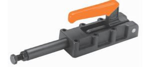
Plunger: Ground Steel. Locks at both extended & retracted ends of the stroke. Base: SG Iron Casting. Body mounting. Nominal Holding Force: 5000 daN Weight: 6.20 Kg Supplied complete with: MB1680 Setscrew & nut. See "Accessories" for other items.
