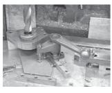
Operating clamping force 500 daN (hand applied), 800 daN (mallet applied). Weight:
