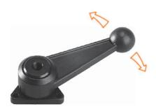
Operating clamping force: 750 daN (hand applied), 4000 daN (mallet applied) Weight: 0.55 Kg
