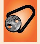
The Pivoting Lifting Ring is a low profile lifting device that pivots 180°. It is one of the most economical lifting devices available and is ideal for applications that do not require a rotating action. This Lift Ring is easy to install and is available in five sizes. Load ratings range from 900Kg - 9,000Kg. The product is manufactured from alloy steel, heat treated and magnafluxed.
