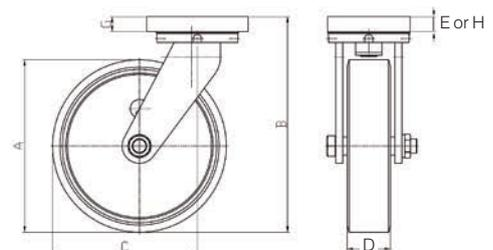
(E) Swivel top plate thickness 26mm
