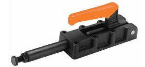
Plunger: Ground Steel. Locks at both extended & retracted ends of the stroke. Base: SG Iron Casting. Body mounting. Nominal Holding Force: 5000 daN Weight: 6.20 Kg Supplied complete with: MB1680 Setscrew & nut. See "Accessories" for other items.
